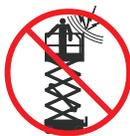
This machine is not electrically insulated and will not provide protection from contact with or proximity to electrical current.
