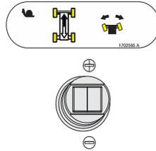
Positioning the steer control thumb operated switch Right or Left enables steering the machine to the right or left respectively.
