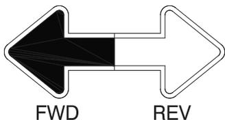
2. Push and release the Drive Orientation Override switch. Within 3 seconds, slowly move the Drive control toward the arrow matching the intended direction of machine travel. The indicator light will flash during the 3 second interval until the drive function is selected.
