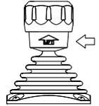
**NOTE:** The Main Boom Lift/Swing joystick is spring loaded and will automatically return to neutral (off) position when released.
