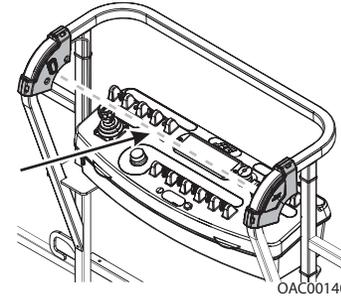
Operator passes through path of sensor beam.
