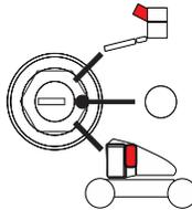
**NOTE:** With Platform/Ground Select switch in the center position, power is shut off to controls at both operating stations.
