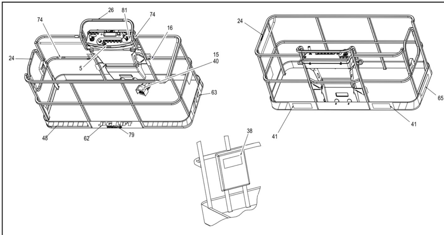
Figure 4-11. Decal Installation - Sheet 6 of 6
