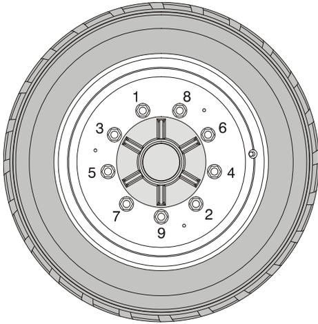
3. The tightening of the nuts should be done in stages. Following the recommended sequence, tighten nuts per wheel torque chart.
